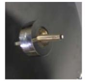
Topside of Weighted Base, with Bolt threaded through 2" Pole Support (tilted to the side)
